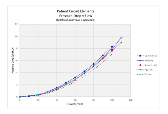
*Figure 3:* Pressure-flow curve of V-Com<sup>™</sup>, 12 mm circuit hose, and 3 nasal pillow masks with small cushions. At high flow (during inspiration) a large pressure drop occurs (reducing IPAP). At low flow (during expiration) minimal pressure drop occurs (preserving EPA
